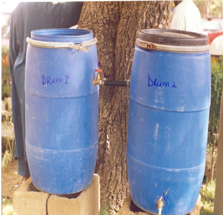
Figure 4. Sand filter drum. Drum 1 (left), sand filter media; drum 2 (right), collection /storage of filtered water.
